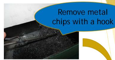
Remove remaining metal chips using a tool
