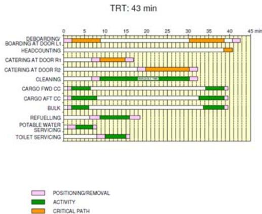
Figure 7: Operations of the turnaround for an A320
